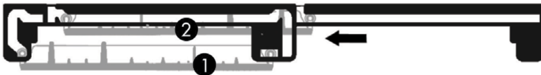
Left rack adjusted to lower position and right rack moved to the left
